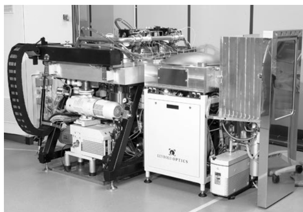
Figure 1: Sputtering tool for the fully automated cleanroom production of optical coatings.
